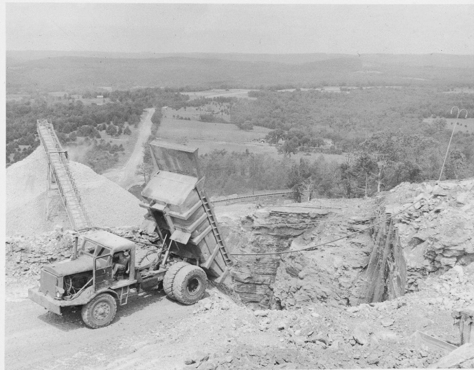
VIEW IN QUARRY, EUCLID TRUCK DUMPING IN CRUSHER CHUTE. AND JIMMY HOFFA?
